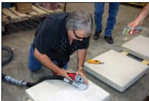
During the certification performance exam, students will need to know how to grind the surface in preparation for a CaCl test.
